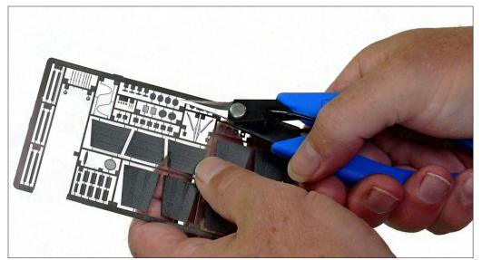
Photo-etched parts add realistic detail to scale models. Because these accessories are delicate and tightly spaced on metal frets, only a precision tool will safely remove them.
